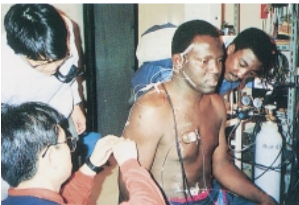
Experiment of thermal sweating in the environmental chamber
