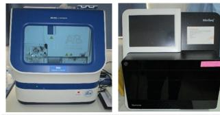
During the fiscal year 2018, the project installed two advanced equipment: a capillary sequencer (ABI 3500, left) and a nextgeneration sequencer (Miniseq, right). These equipment will reinforce the research capabilities at CERMEL.
